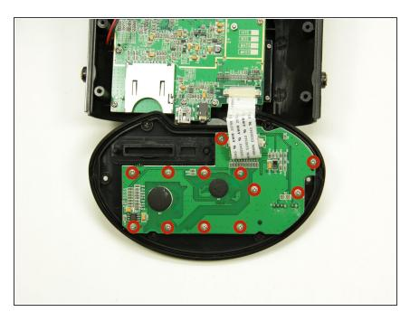
Using a Philips head screwdriver, remove the 12, 3mm screws from the board.
