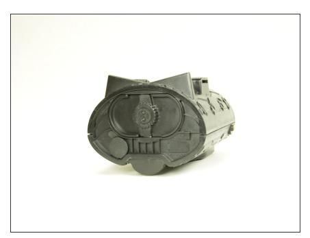
Grabbing the knob, turn it counterclockwise until the latch is out of it's groove.
