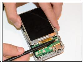
Use a spudger to carefully detach the ribbon cable without breaking it.
