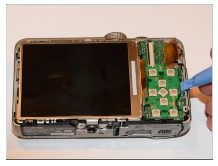
Use the plastic opening tool to lift and remove the buttons board as shown.
