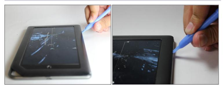
• Pry off the front panel using the plastic opening tool.
