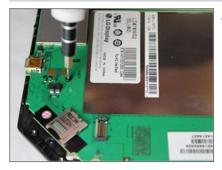
• Remove the easy-to-miss T5 Torx 3.8 mm screw located in the tabbed corner of the device.
