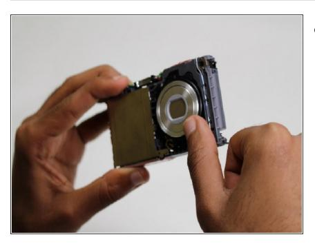
Pop out the lens zoom unit from the frame by using either your thumb or an opening tool.
