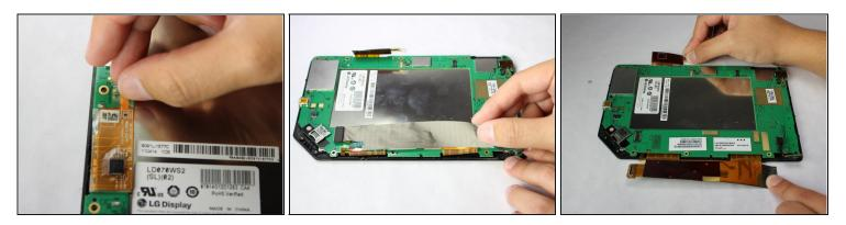
• Gently lift and peel the orange and grey ribbon connectors to disconnect the screen and motherboard.
