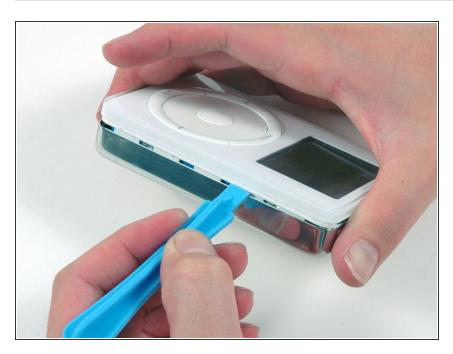
Free the five tabs holding the iPod together on the other side. You may be able to free the tabs by gently wiggling the front panel of the iPod.
