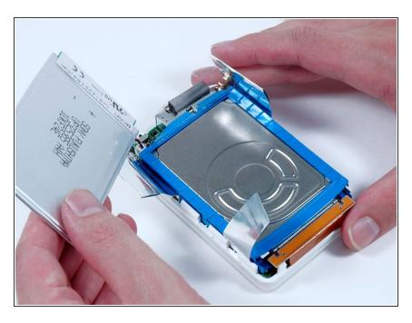
Lift the battery up from the hard drive and lay it next the the iPod (it is still connected to the logic board).
