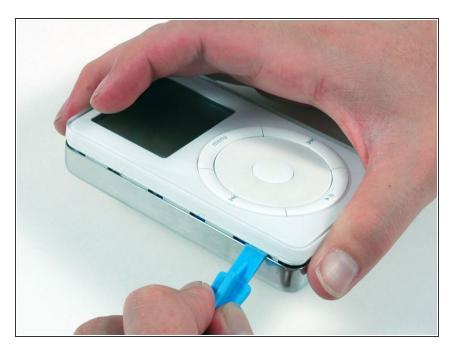
Continue to run the opening tool along the side of the case until all five tabs have been released.
