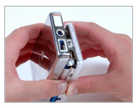
Lift the rear panel away from the iPod, making sure it doesn't catch on the headphone jack.
