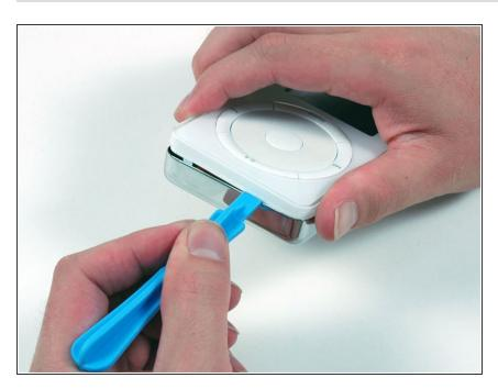
Work around the corner of the iPod and release the two tabs holding the iPod together near the dock connector.
