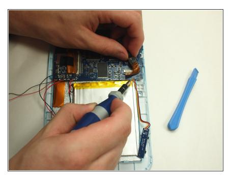
Un-solder the yellow, red, and black wires that connect the volume module to the motherboard.
