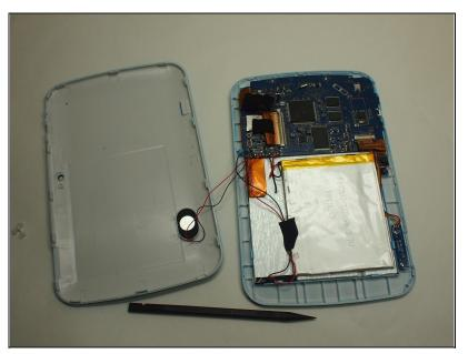
Locate the red and black wires that connect the speaker to the motherboard.
