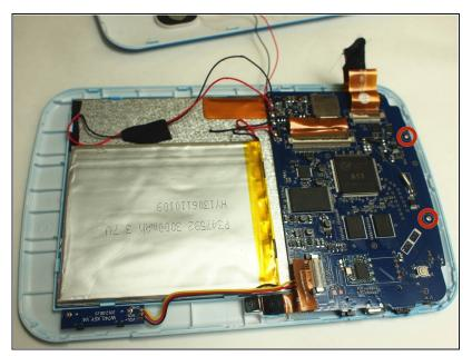
Remove screws located on the opposite side of the battery.
