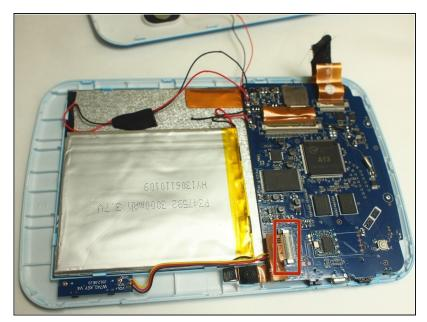
Use the precision <u>tweezers</u> to gently disconnect the camera ribbon that is connected to the motherboard.
