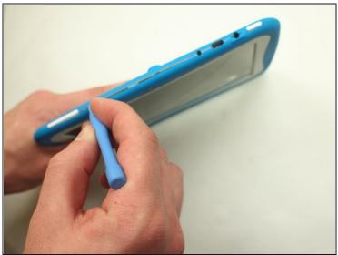
• Slide the wide plastic opening tool across the seem, separating it if you can't pry the device open using just the spudger.
