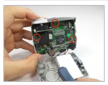
Remove the four screws from the motherboard.
