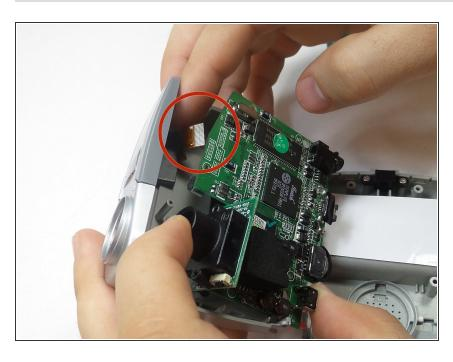
Take out the motherboard while disconnecting the flip screen's cable from underneath.
