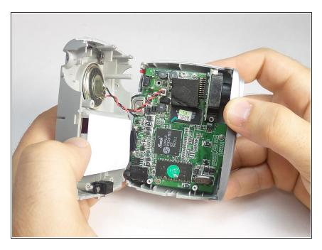
Unfold the device and be careful not to tear the black and red power supply wires.
