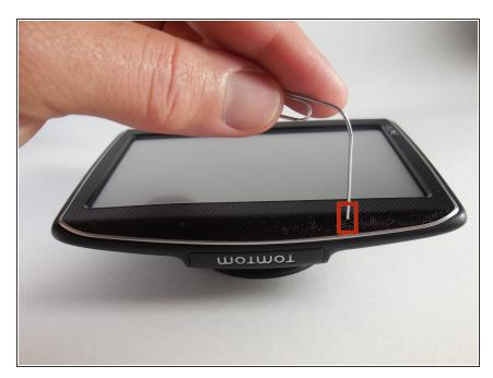
The reset button is located at the top of the device, close to the charging port. It is a small hole that is .78 mm wide.
