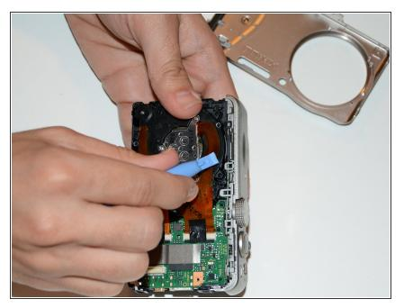
• Remove the top cover using the plastic opening tool.
