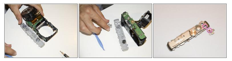
• After removing the top cover of the camera, you will be able to easily remove the power button with your hand.
