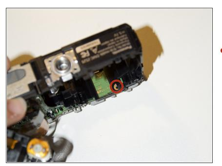
To release the top cover of the camera, you need to open the 3.70 mm screw shown in the picture.
