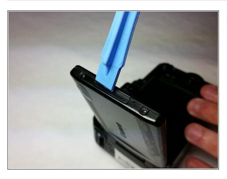
Use the plastic opening tool on the indent at the top of the LCD screen to pop off the LCD case.
