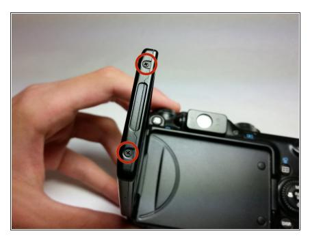
Remove the two 3.10mm Phillips #00 screws from the LCD case.
