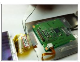
• Use the tweezers to lift the small brown plastic snap before you remove the wire.
