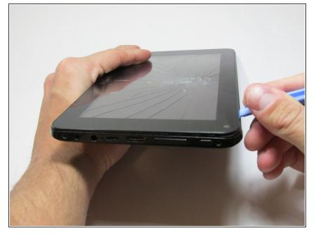
Using a plastic opening tool, work your way around the edge of the device, separating the case from the rest of the device
