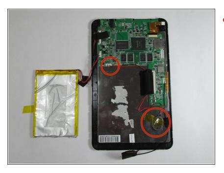
Identify the connection location of the wires from the speakers.
