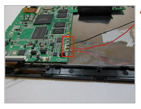
Solder the new speakers to the correct location, making sure the red wire goes to the + and the black wire goes to the -.
