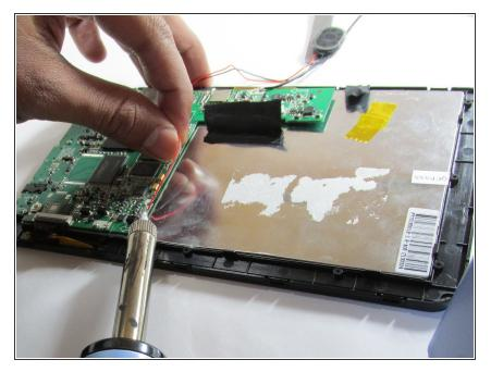
• Use a soldering iron to remove the speaker wires from the circuit board
