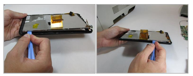
• Using the plastic opening tool, begin separating the front screen from the display
