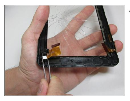
Once screen has been separated, use tweezers to remove front camera
