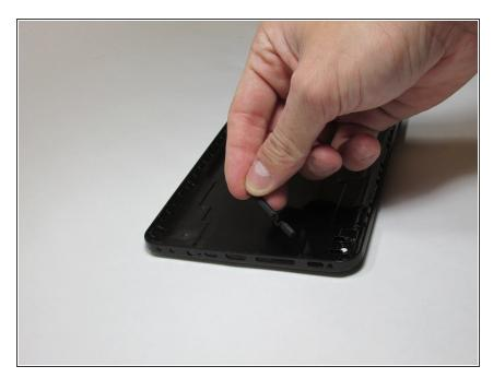
Remove the black buttons (they should not be directly attached to the device and may fall out).
