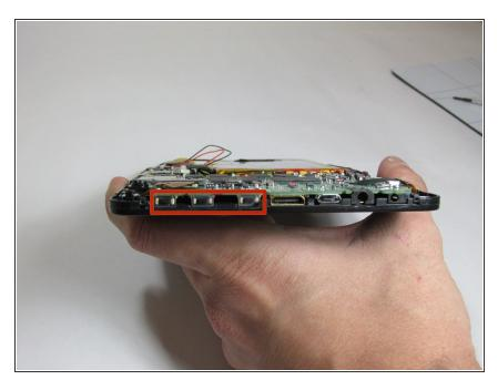
On side the circuit board there will be three buttons. One is the power button, and the other two are volume buttons.
