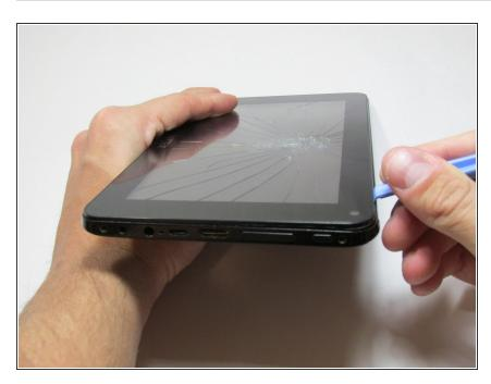
Using a plastic opening tool, work your way around the edge of the device, separating the case from the rest of the device
