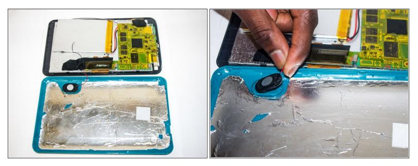
• Carefully peel the tape holding down the wires connected to the speaker.
