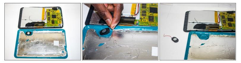
• Remove the speakers by using your hand to entirely disconnect the back cover.
