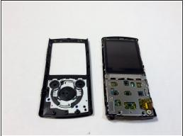
Using a plastic opening tool, work your way around the edges of the device, carefully prying off the front panel.
