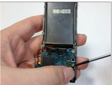
Peel back the ribbon for the audio jack and remove the 1.8mm silver Phillips screw.
