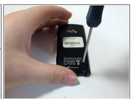
Remove the two black 6.4mm Phillips screws from the back of the device.
