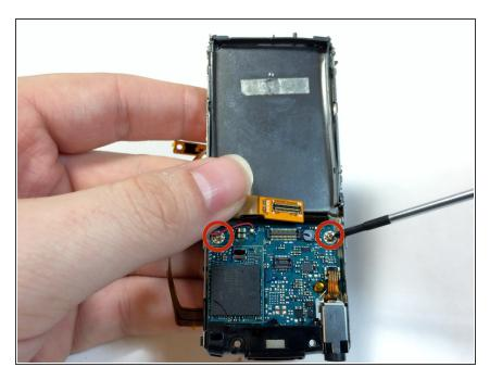
Lift up on the LCD ribbon and remove the two 1.8mm silver Phillips screws.
