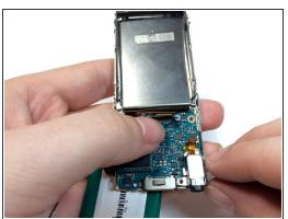
Use the flat end of a spudger to flip up the retaining flap on the audio jack module.
