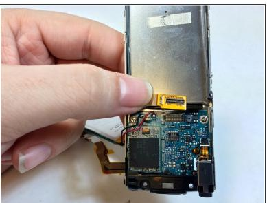
Use the prying tool to remove the LCD ribbon wire.
