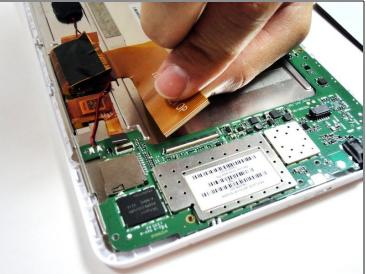
• Remove the larger ribbon cable by gently flipping the beige latch and pulling it out with tweezers.
