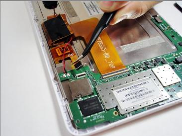
• Remove the smaller ribbon cable by gently flipping the black latch and pulling it out with tweezers.
