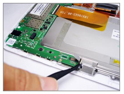
Gently pry the front facing camera plug up and off of the motherboard.
