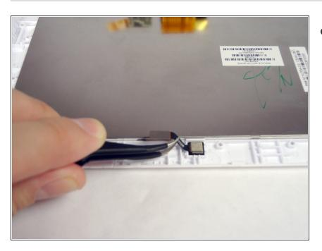
Gently remove the camera from the device with tweezers by lifting it up and out of its square hole.
