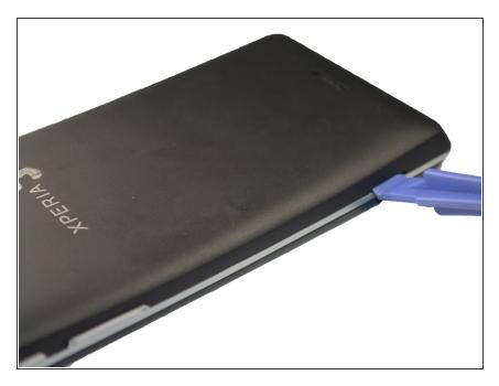
Find the little bracket on the bottom left of the phone (when looking at it upside down) and use the opening tool to pry off the back cover.
