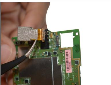
Pop the camera out using your fingers, and then unclip it off the board using tweezers.
