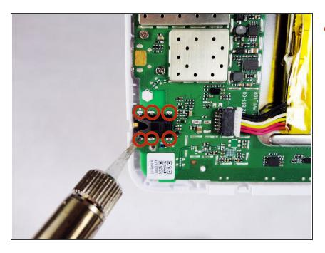
Desolder the top lead for the six solder points.
