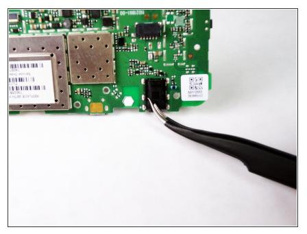
• Once the solder is removed, gently pull the audio jack away from the motherboard with tweezers.
