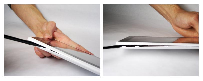
• Use a Spudger to open the back panel. Be careful not to break the tabs.
