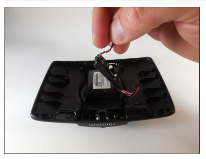
Simply lift the speaker up and out of the base to replace it.
