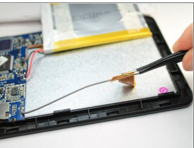
Gently peel the WIFI Antenna up using a pair of tweezers.
