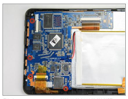
Remove the four 2.2mm Phillips screws holding the logic board in place. Place the screws on the iFixit magnetic project mat.
