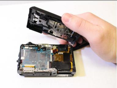
Separate the front and back housings carefully.
