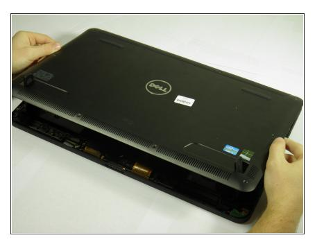
Gently lift the back cover off the device. The back cover should come off easily.
