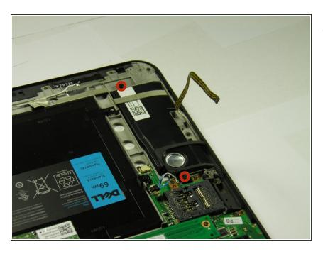
Remove the two black 4mm screws with a Phillips 00 screwdriver.
