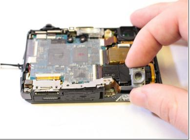
Remove the tripod receptacle by simply lifting it out with your hands or with tweezers if necessary.
