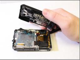
Gently lift the front panel up off the back of the camera prying up around the edges using a plastic opening tool or spudger if necessary.
