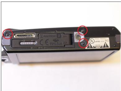
Remove all seven black 4 mm Philips #00 screws holding the front panel into place. Two on each
