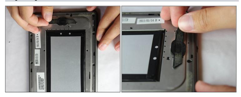
Remove the protective lining located above the speaker.
