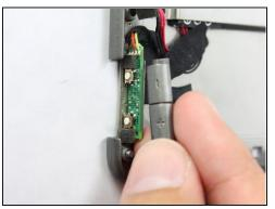
• Once you have removed both the back and front panels of the device, you will isolate the panel which contains the buttons. You will remove the volume buttons on the top right first. Use some force upwards and the button will slide free.
