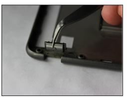
Next, you will remove the power button from the top left of the middle portion of your device. Using tweezers you will carefully lift the button from where it sits and remove it.
