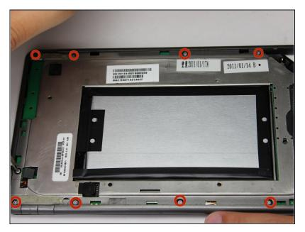
Remove the ten 4.0 mm screws from the device's perimeter using the T5 Torx screwdriver.
