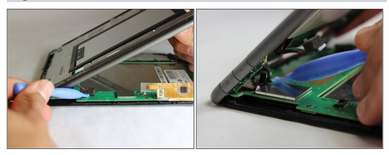
• Lift up on the connectors to disconnect them using the plastic opening tool.
