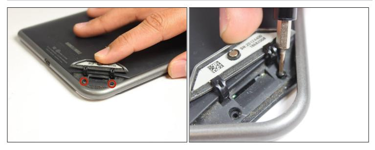
• Remove the two 3.8 mm screws located in the back right corner of the device using the T5 Torx screwdriver.
