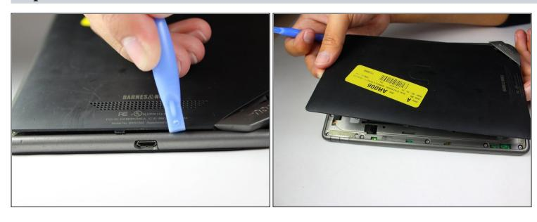
• Pry off the back cover with the plastic opening tool. Go around the device with the tool to ensure complete detachment.
