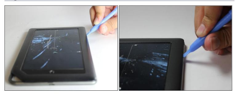
• Pry off the front panel using the plastic opening tool.
