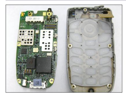
• The motherboard should now be completely removed from the phone.
