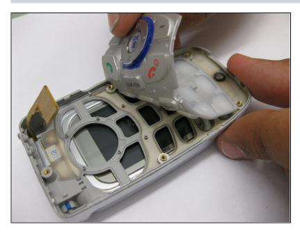
• Once the motherboard has been removed, peel the keyboard as pictured.
