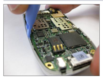
Using a spudger, lift the motherboard out of the phone case as pictured.
