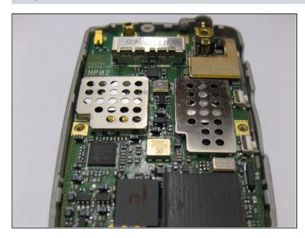
• The back case should now be completely removed and the motherboard will be visible.
