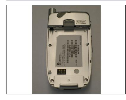
• The back of the phone will look like this when the battery is correctly removed.
