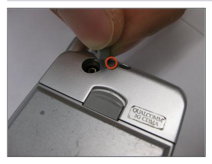
• Remove the screw that sits underneath the rubber covering.
