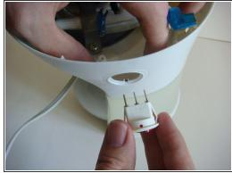
Gently squeeze the sides of the Power Switch, while using a Spudger to help pop out the Power Switch.
