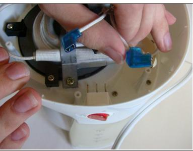
Using a Plastic Opening Tool, carefully slide back the three power connectors for the Power Switch until fully removed.
