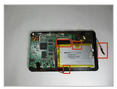
Remove the yellow and black tape around the battery very carefully
