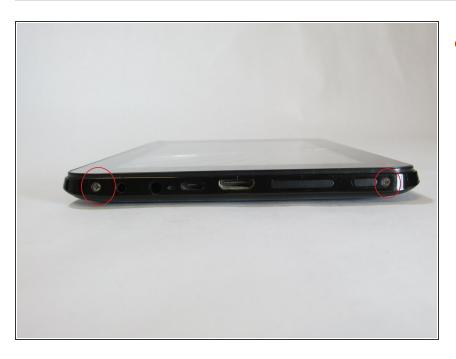
Using a small phillips screwdriver, unscrew both end screws
