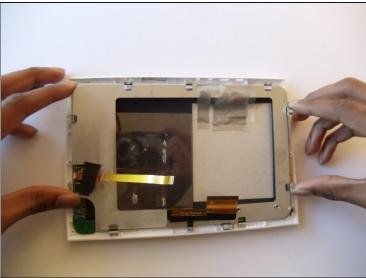
Slowly remove the metal frame and screen from the white casing by gently pulling up on the ends of the metal frame.
