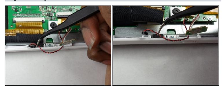
• Use your <u>tweezers</u> to gently remove the microphone from the slot in the casing.
