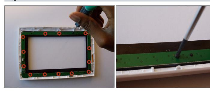
• Unscrew each of the 14 black, phillips #00 (3mm x 3mm) phillips head screws from the screen sensor.
