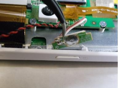
• Use a tweezer to gently pull the power button sensor out of the case's slot.
