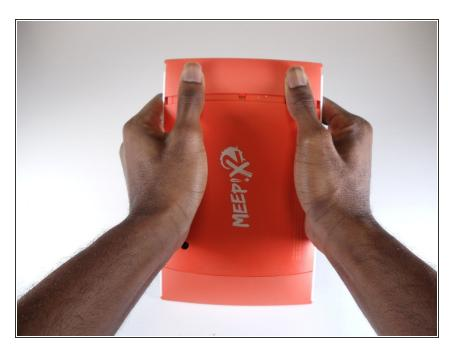
Remove the orange covers from the left and right sides of the device by sliding up against the tabs.
