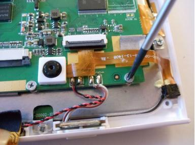
• Remove the two phillips #00 (4.5mm x 3mm)screws located on the motherboard.
