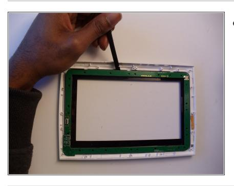
Use the spudger to gently undo the sensor from the white casing.
