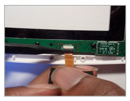
Use the spudger to undo the ribbon cable security clip located on the far left of the screen sensor.
