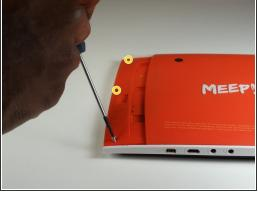
You can remove the rear casing by unscrewing all six phillips #00(3.5mm x 4.5mm)screws from the left and right side of the device.
