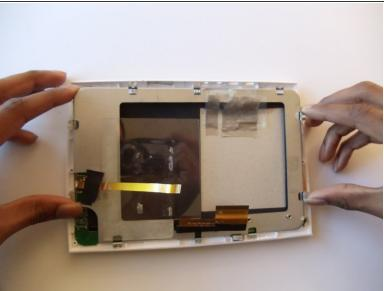
Slowly remove the metal frame and screen from the white casing by gently pulling up on the ends
