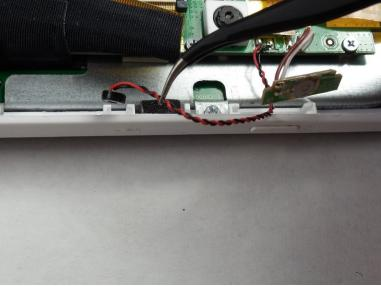
• Use your tweezers to gently remove the microphone from the slot in the casing.
