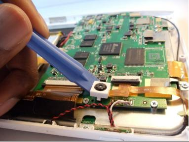
Slip the plastic opening tool under the white, square enclosure of the camera and lift upward to unhook the camera unit from the motherboard.
