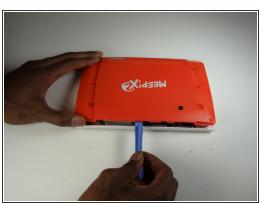
Use the plastic opening tools to undo the clips around the edges of the device.
