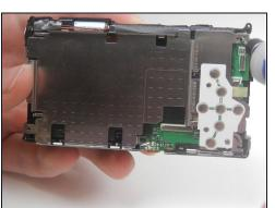
Unscrew the two 3.5 mm Phillips head screws in the metal plate.
