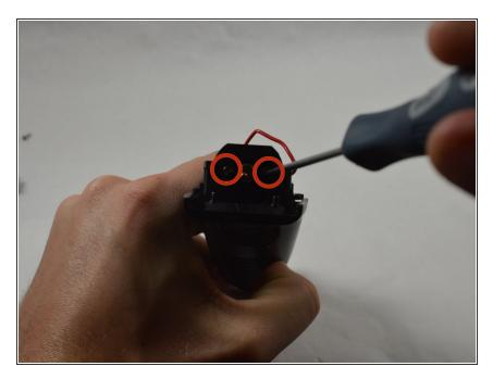
Remove two 3.0 mm PH00 screws from the plastic housing.
