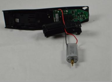
Remove the motor by carefully prying on the back side of the motor with a spudger.
