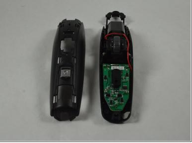
Remove the two 11.0 mm PH00 screws that attach the zoom wheel to the plastic housing.
