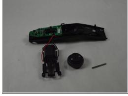
A pin holds the wheel in place. Using a spudger (preferable metal) and a pair of pliers or tweezers remove the pin to unseat the wheel.
