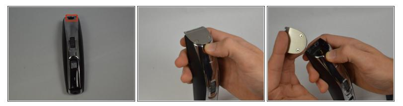
Press the black button below the blade to remove the blade.
