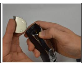
Press the black button below the blade to remove the blade.
