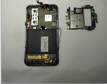
Use a spudger or pair of tweezers to grab the top left corner of the motherboard and gently lift it out, taking care to not damage any of the ribbon cables when removing. To reassemble your device, follow these instructions in reverse order.
