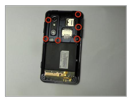
Remove the six Phillips #00 screws within the mid-cover bezel.
