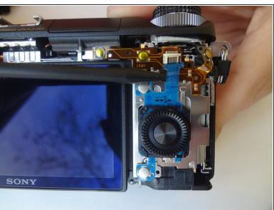
Pry out the ribbon cable by carefully pushing on its side tabs with a spudger.
