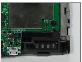
Use the pointy end of your Spudger to separate the Speaker's connector from the motherboard on both sides.
