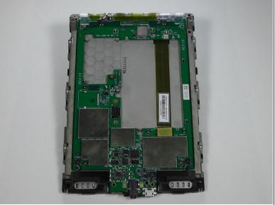
With the screws removed, gently remove the case from the internals.
