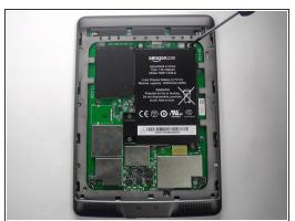
Use a Phillips #00 screwdriver to remove the five screws.
