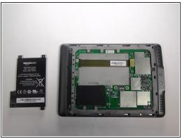
Using the flat end of your spudger, gently pry the battery up and remove it.
