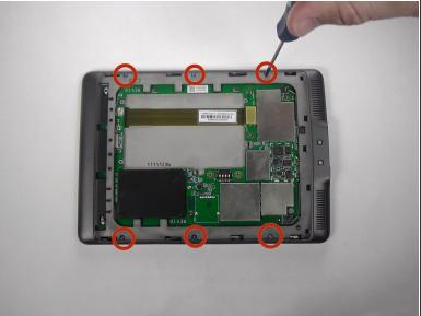
• Using a Phillips #00 screwdriver, remove the six 4 mm screws to access the front plate.
