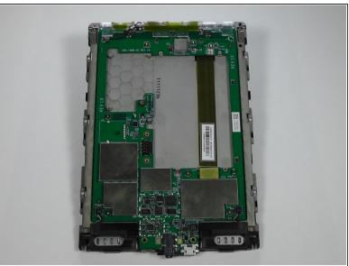
With the screws removed, gently remove the case from the internals.
