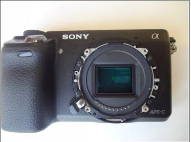
To remove the inner lens mount ring, remove the two silver 2.0 mm Phillips #00 screws. This will complete the removal of the lens mount.
