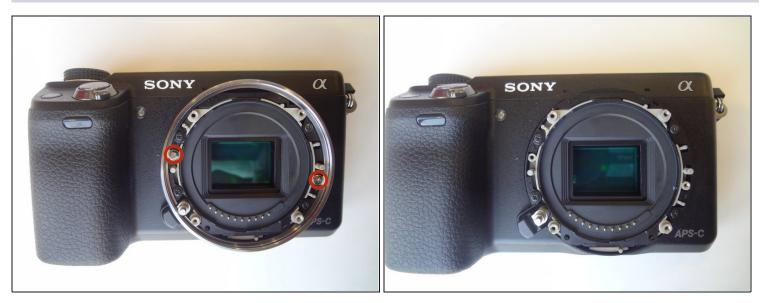
• To remove the inner lens mount ring, remove the two silver 2.0 mm Phillips #00 screws. This will complete the removal of the lens mount.
