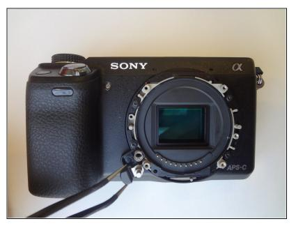
By using tweezers, carefully remove the lens-release button by lifting upward.
