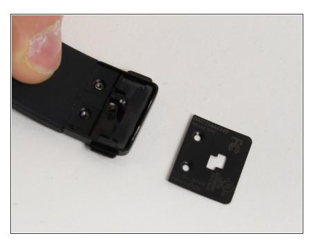
Remove the metal plate with the serial and model number on it by pulling it straight up around the two hooks.
