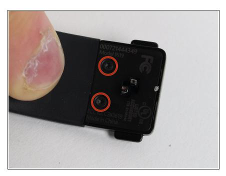
Using the T3 Torx Screwdriver, remove the two 2.00mm long screws from the inside of the clasp.
