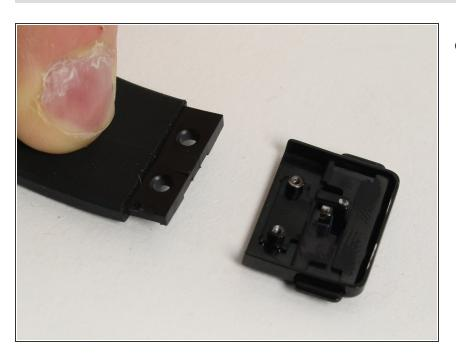
Pull the two securing pins out of the rubberized part of the band.
