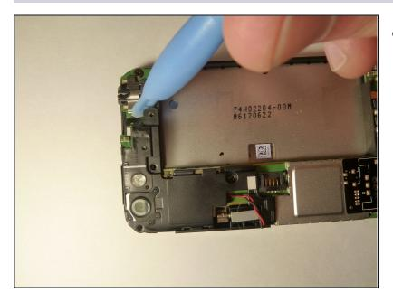
Pry off the camera lens using a plastic opening tool.
