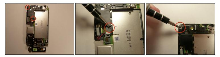
• Remove the two 3.0 mm Phillips #0 screws, that are securing the camera lens.
