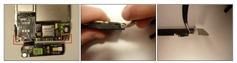
• Using <u>tweezers</u>, pull back on the tape located on the bottom corners of the motherboard.
