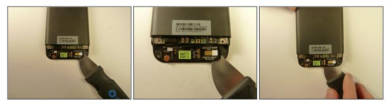
Use a Jimmy to pry up the OEM SIM and SD card reader contact.
