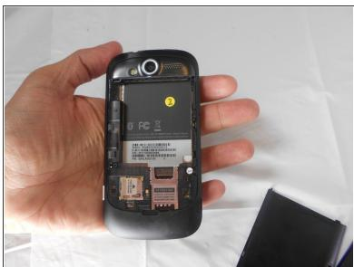
Use the plastic prying tool in the upper left-hand corner notch of the battery to remove.
