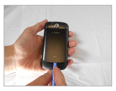
Place the prying tool into the notch at the bottom of the case and pull up to remove.
