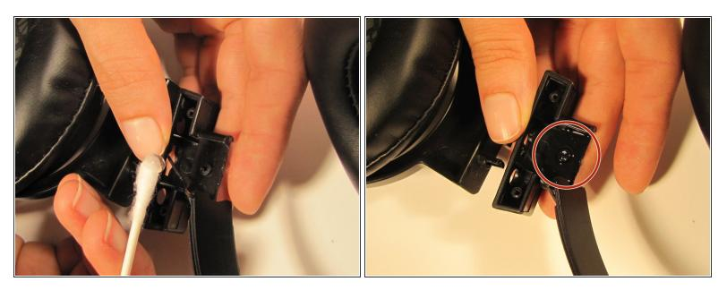
• Cover the detached slider port in a generous layer of Plasti Dip, which works like glue. Also coat any exposed wire to seal the circuit.
