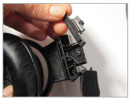
• Remove the bottom inner casing to reveal the wire compartment and the port where the slider inserts.
