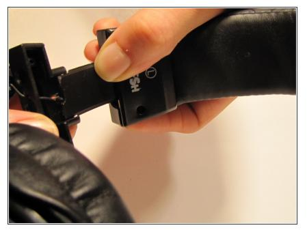
Realign the broken size adjuster into the port with the Plasti Dip so that it can be secured to the ear piece.
