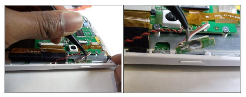
• Use a tweezer to gently pull the power button sensor out of the case's slot.
