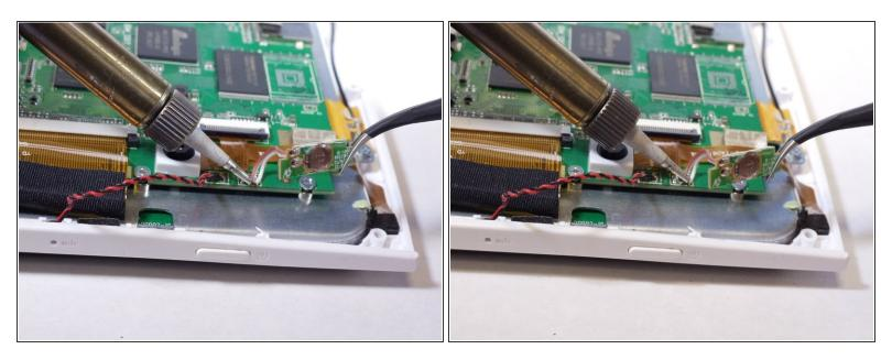
• Use the soldering station to unsolder and remove the power button from the motherboard.
