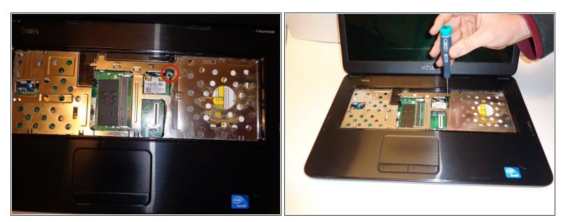
• Locate and remove the 4mm Phillips #00 mounting screw.
