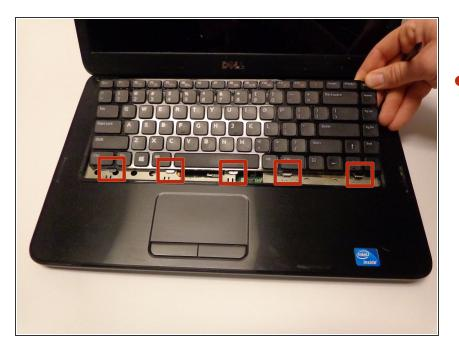
Slide the keyboard forward towards the screen to release the bottom tabs.
